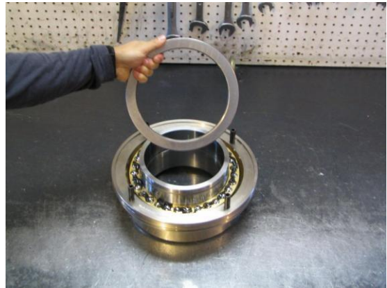
Put a bead of grease on the bearing, and then install the outer race with the smallest bore.
