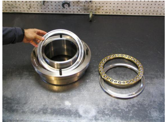
Install the outer race with the largest bore first.
