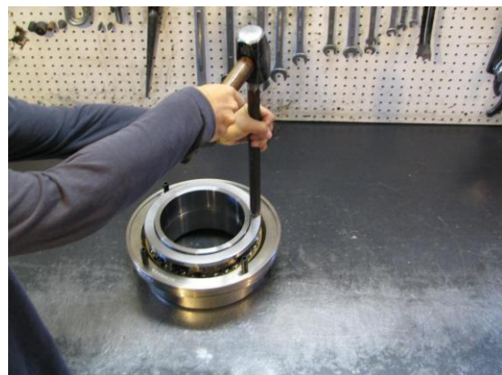
The 2 nd outer race must be hammered on.
