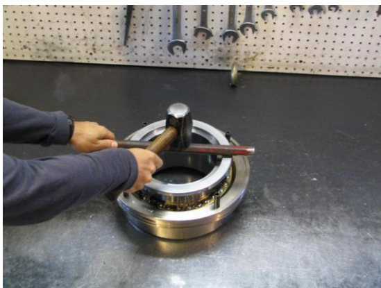
The 2 nd outer race must be hammered on.
