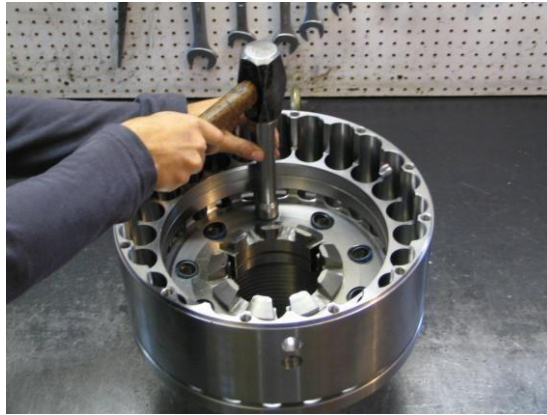
Insert the 9 Oil Seals (18100439) in the Chuck Housing (18100438).
