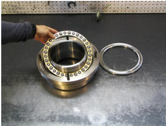
Put a bead of grease in the outer race, and then install the bearing cage.
