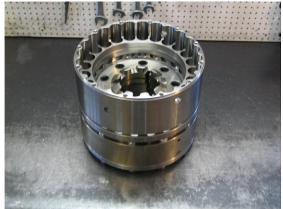
Insert the 9 Oil Seals (18100439) in the Chuck Housing (18100438).
