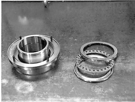
Install the 3 part bearing.
