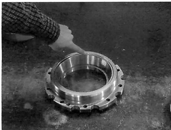
The bearing cup must bottom out in the Bearing Retainer
