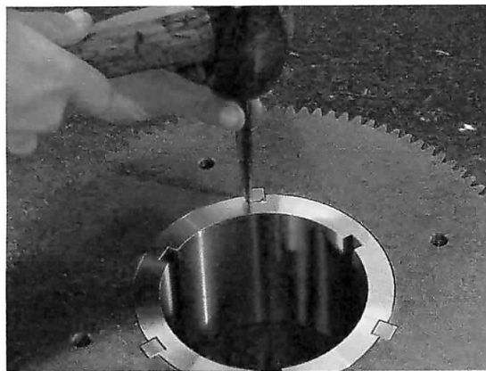
Punch the edge of the key and the drive sleeve to ensure that the keys do not fall out
