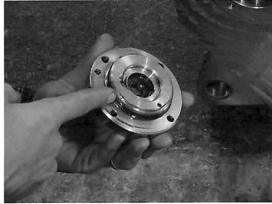
Apply grease to the outside of the Mounting Adapter.
