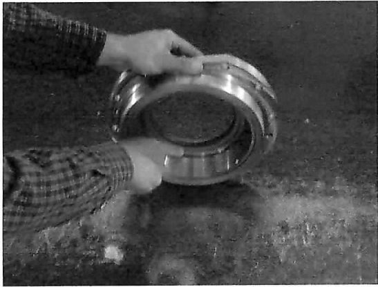
The oil seal must bottom out in the Bearing Retainer
