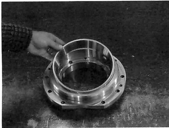
Install the bearing cup in the Lower Bearing Retainer (18100237). The cup can be pressed or hammered into place.
