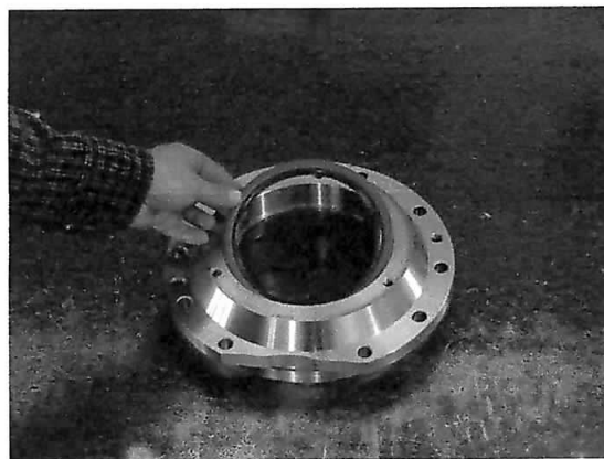
Flip the Bearing Retainer over and install the first Oil Seal (18100351). Spring facing down.
