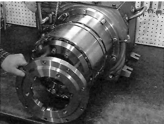
Install the Top Cap Holder (18100122) and torque the 9 bolts (1/2" x 2 1/4" long) to 70 ft.lbs.
