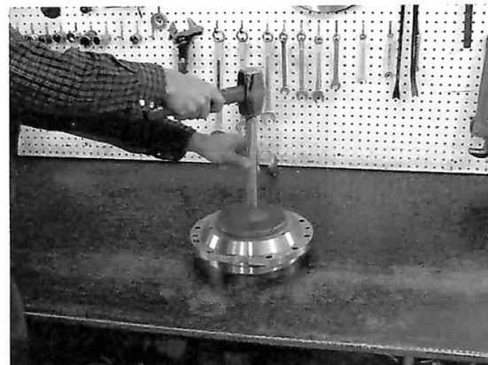
Hammer the oil seal into place
