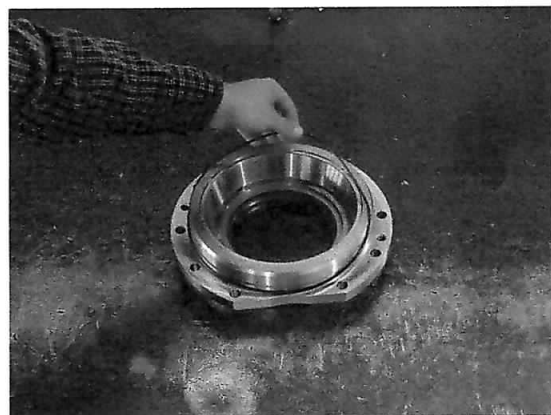
Flip the Bearing Retainer over and install the O-Ring (18100350).
