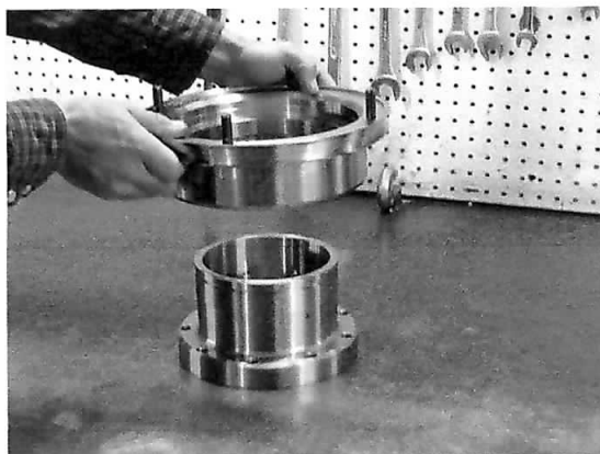
Place the piston over top of the actuator sleeve (18100123)
