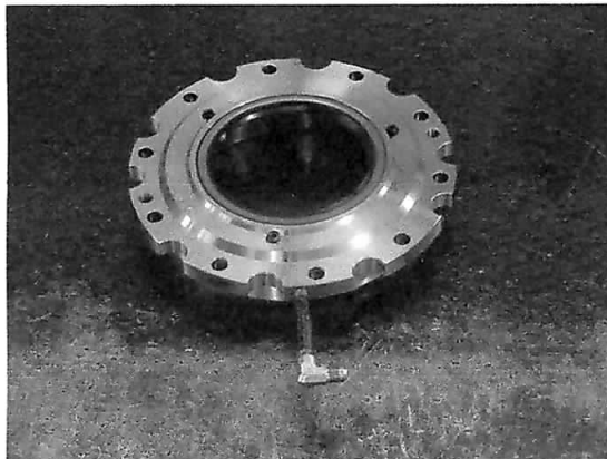
Insert the 3" long pipe nipple and 90 deg. fitting as shown
