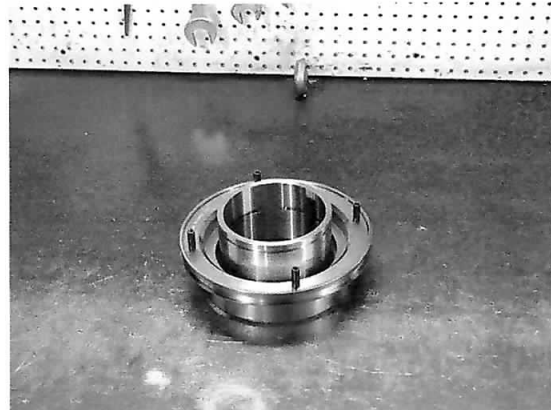
Place the piston over top of the actuator sleeve (18100123)
