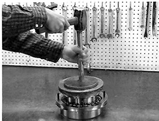
The 2 nd outer race must be hammered on.
