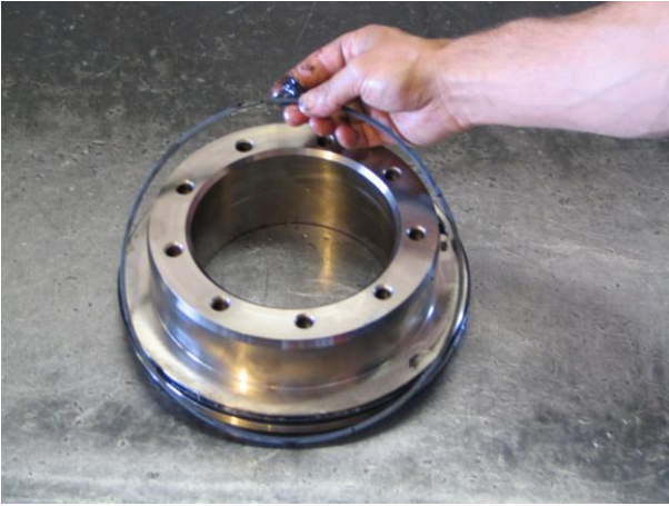
Apply grease to the Wear Ring (18100063) and install it in the bottom groove of the Piston.
