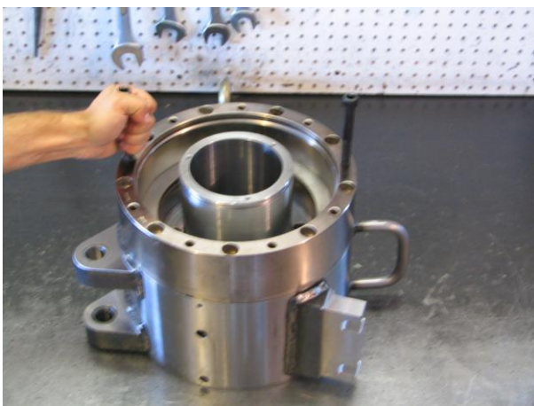
Install the Cylinder (18100052) on the Rod Clamp Housing (18100170) (you can use 2 bolts as shown to assist you). NOTE the position of the ¼ NPT tapped hole on the side of the Cylinder.
