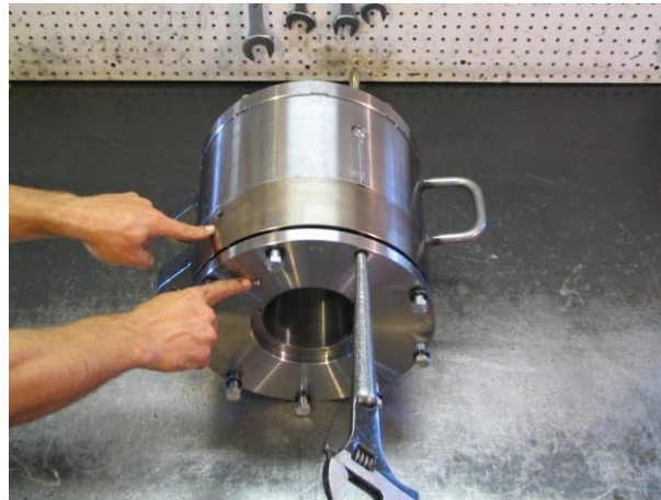
Install the Bottom Cap in the Cylinder.
