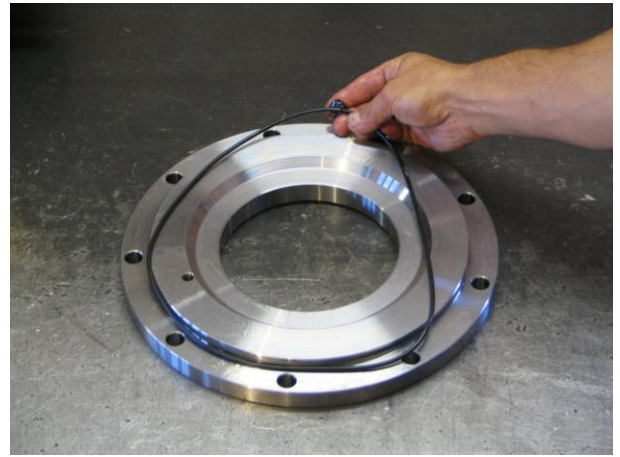
Install the O-Ring (18100192) in the Bottom Cap (18100172).
