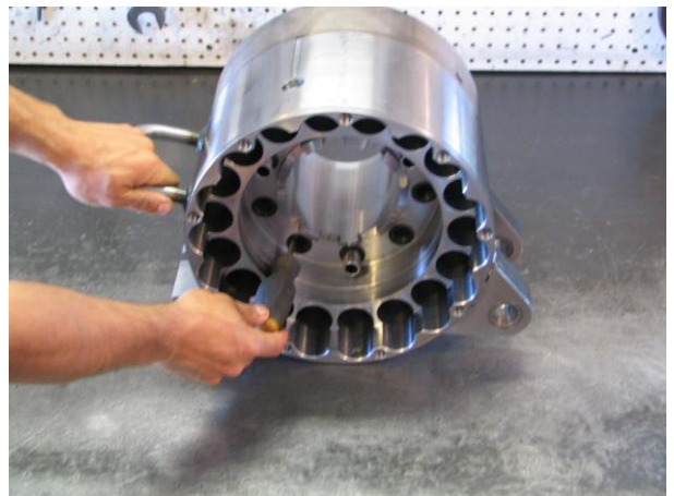
Properly align the 9 tapped holes in the Piston with the holes in the Clamp Housing
