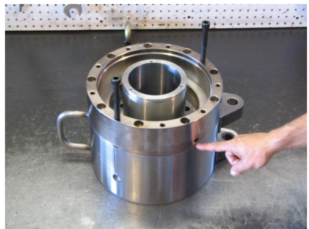
Install the Cylinder (18100052) on the Rod Clamp Housing (18100170) (you can use 2 bolts as shown to assist you). NOTE the position of the ¼ NPT tapped hole on the side of the Cylinder.
