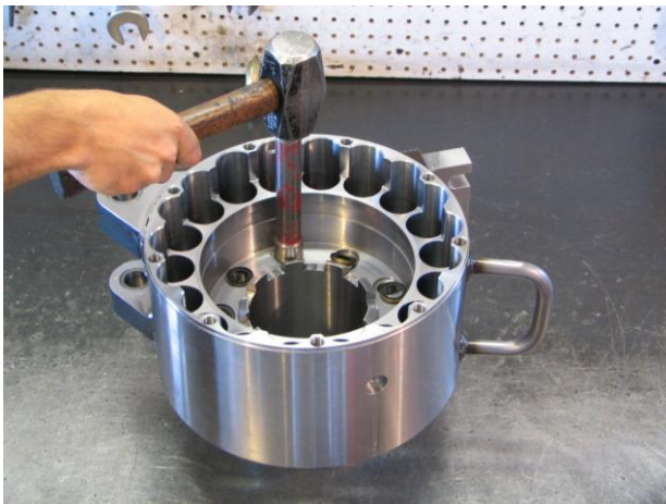
Install the 9 Oil Seals (18100156) in the Rod Clamp Housing (18100070).
