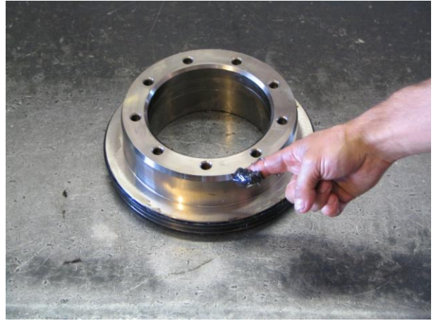
Apply grease at the top of the Piston, to facilitate the installation in the Cylinder.
