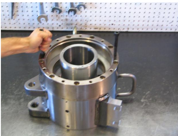
Install the Cylinder (18100052) on the Rod Clamp Housing (18100070) (you can use 2 bolts as shown to assist you). NOTE the position of the ¼ NPT tapped hole on the side of the Cylinder.
