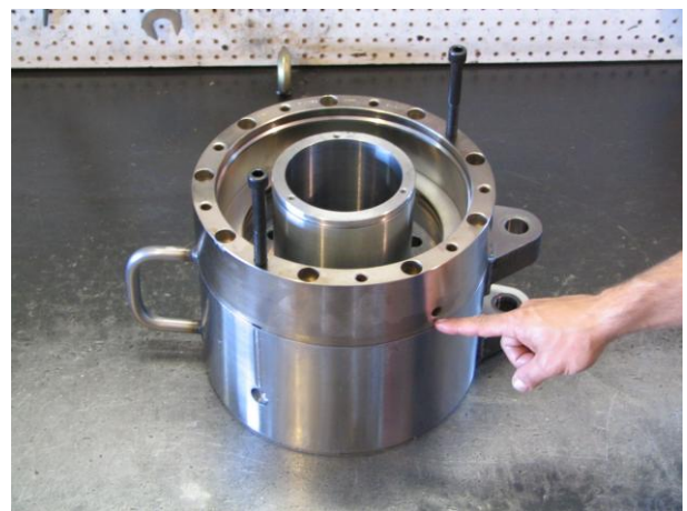
Install the Cylinder (18100052) on the Rod Clamp Housing (18100070) (you can use 2 bolts as shown to assist you). NOTE the position of the ¼ NPT tapped hole on the side of the Cylinder.
